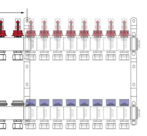
The manifold can either be used as a standalone setup, or can be adapted with a Warmup WHS-M-S3-MIX mixing unit providing regulated temperature control enabling tailored system performance.
